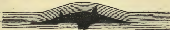
FIG. 11.—Diagram to illustrate the formation of a dome-shaped uplift caused by the intrusion of lava.
